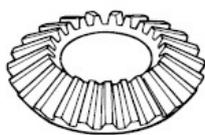
A simple form of bevel gear having straight teeth which, if extended inward, would come together at the intersection of the shaft axes.
