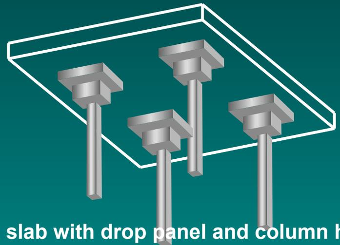
Flat slab with drop panel and column head
