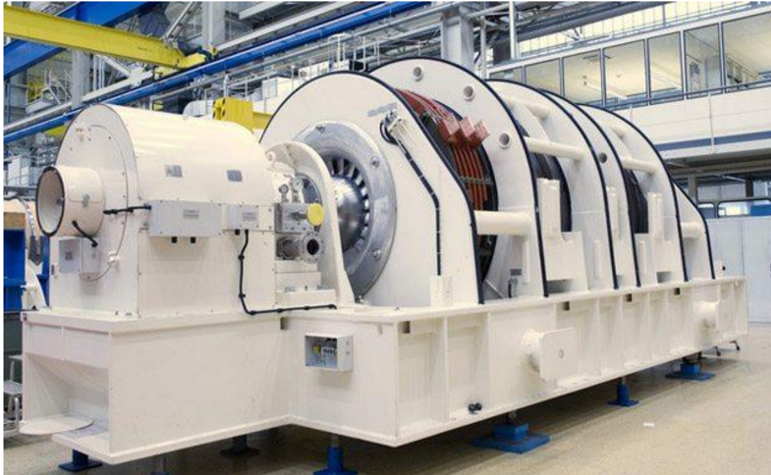
SIEMENS's 2 pole generators customized for the use on gas and steam turbines
