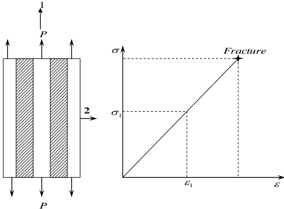
**Fig.1.4 Unidirectional lamina loaded in the fiber-direction**
