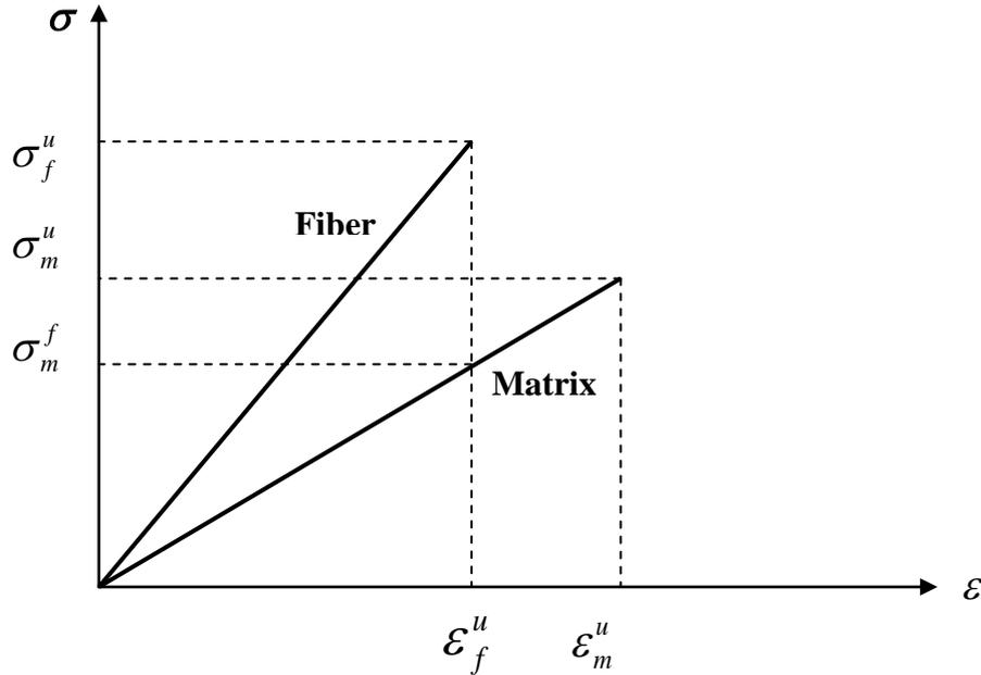
**Fig .1.2 Stress-strain relationships for fiber and matrix**
