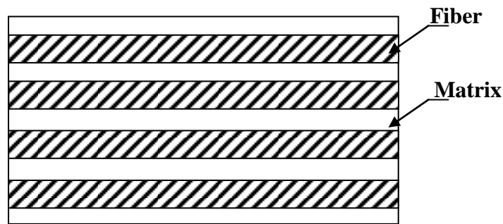
Fig. 1.1 Structure of a fibrous composite
