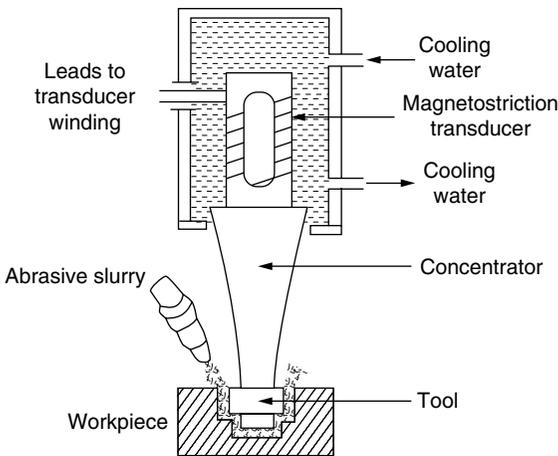
Figure 2.2 Main elements of an ultrasonic machining system.
