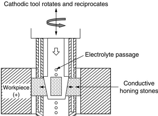
Figure 6.7 ECH schematic.
