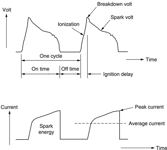
Figure 5.4 Voltage and current waveforms during EDM.
