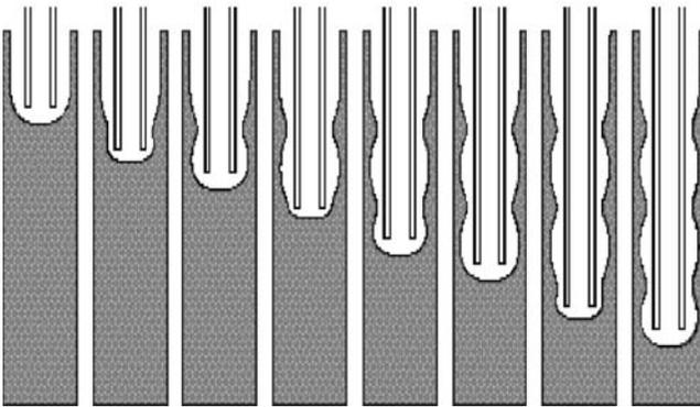
**Figure 4.24** Turbulated cooling holes produced by STEM ([www.win.tue.nl/](http://www.win.tue.nl/)).
