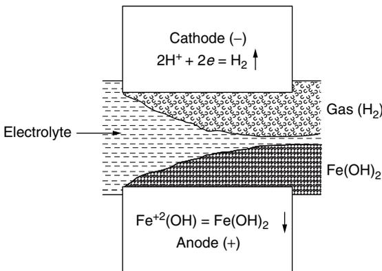
Figure 4.1 Electrochemical reactions during ECM of iron.
