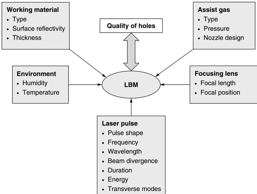
**Figure 5.37** Parameters affecting the quality of laser-drilled holes.
