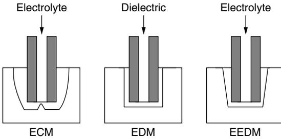
Figure 7.11 Holes drilled by ECM, EDM, and EEDM.
