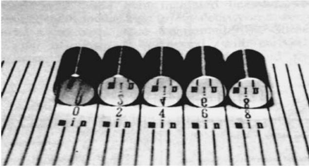
**Figure 6.17** Specimens polished by ECB (Hoshino et al. 1995).
