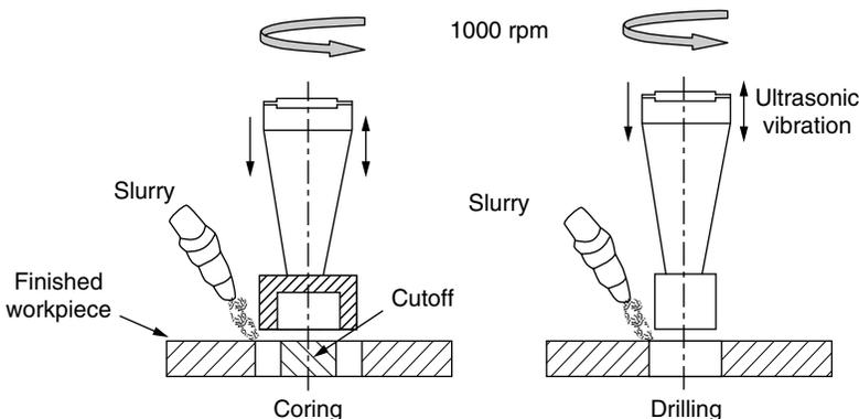
Figure 2.12 Rotary USM.
