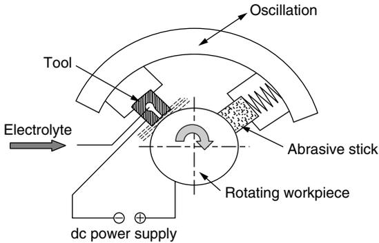
**Figure 6.11** Superfinishing using separate EC electrode (Youssef, 1971).
