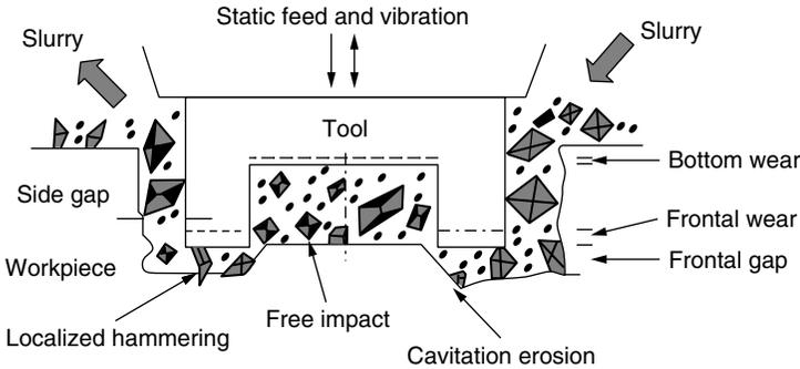
**Figure 2.10** Material removal mechanisms in USM (Thoe et al., 1995).
