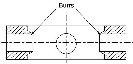
Figure 4.29 Burrs formed at intersections of holes.
