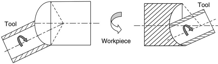
Figure 5.18 Rotary EDM.
