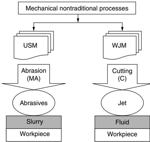
Figure 1.6 Mechanical machining processes.
