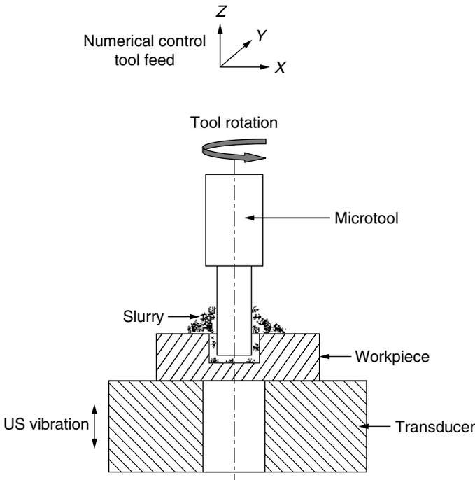
**Figure 2.17** Micro-ultrasonic machining.
