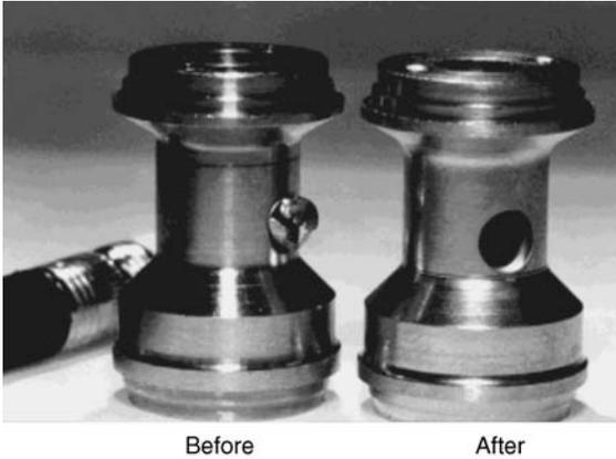
**Figure 4.33** EC deburring applications ([www.extrudehone.com/cation](http://www.extrudehone.com/cation)).
