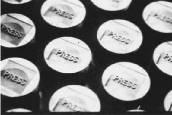
**Figure 2.15** Graphite EDM electrodes machined by USM (Gilmore, 1995).
