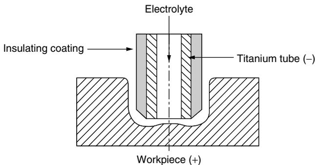
Figure 4.23 STEM schematic.
