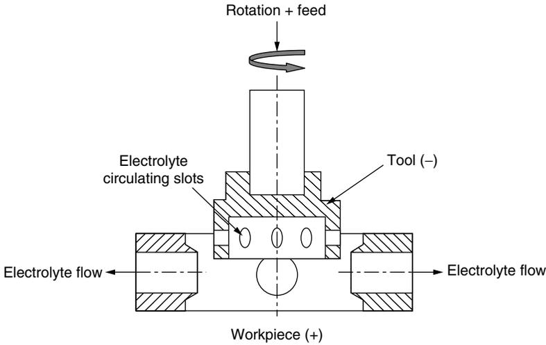
**Figure 4.32** Electrochemical deburring using a rotating tool.
