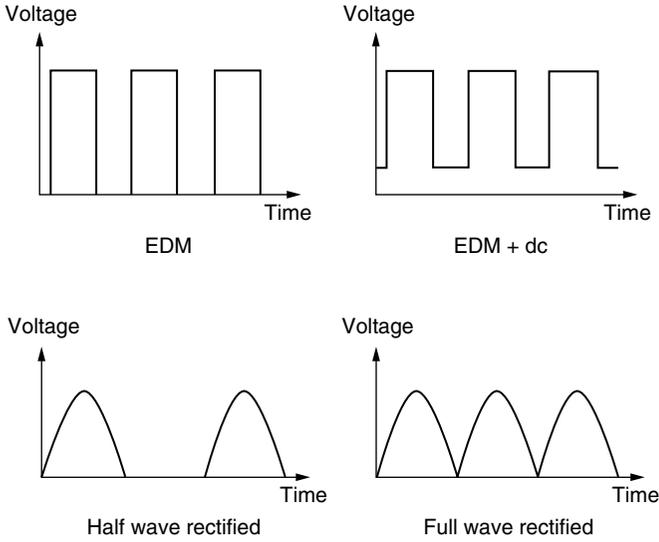
Figure 7.5 Voltage waveforms.
