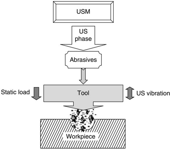
Figure 2.1 USM components.
