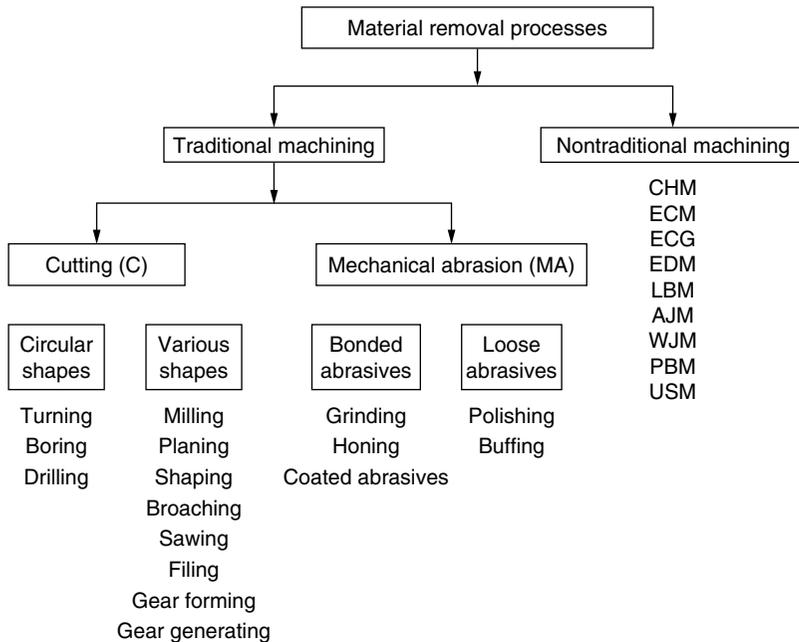
Figure 1.2 Material removal processes.
