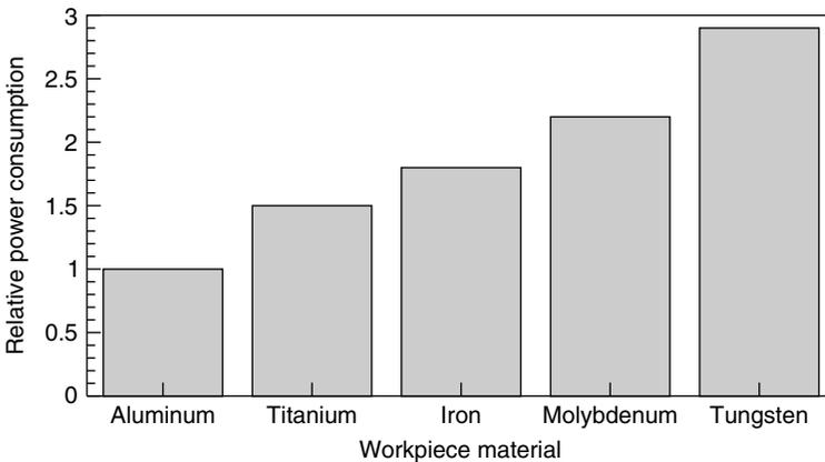
**Figure 5.46** Relative power consumption for different materials (El-Hofy, 1995).
