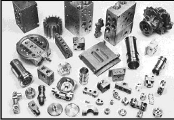
**Figure 4.30** Different components that require deburring (www.vectron.cc/).
