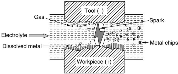
**Figure 7.7** Surface formations in EEDM (El-Hofy and Khayry, 1995).
