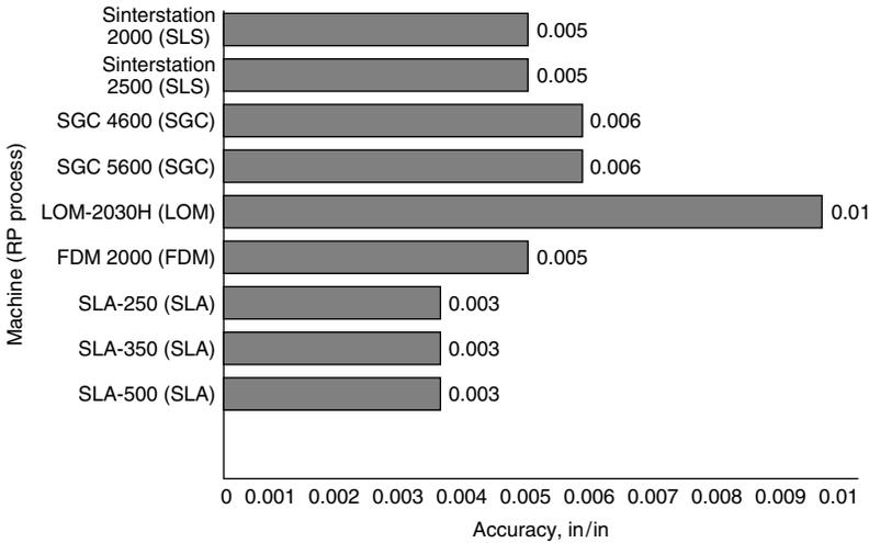
Figure 8.14 Accuracy levels for RP techniques (Wright, 2001).
