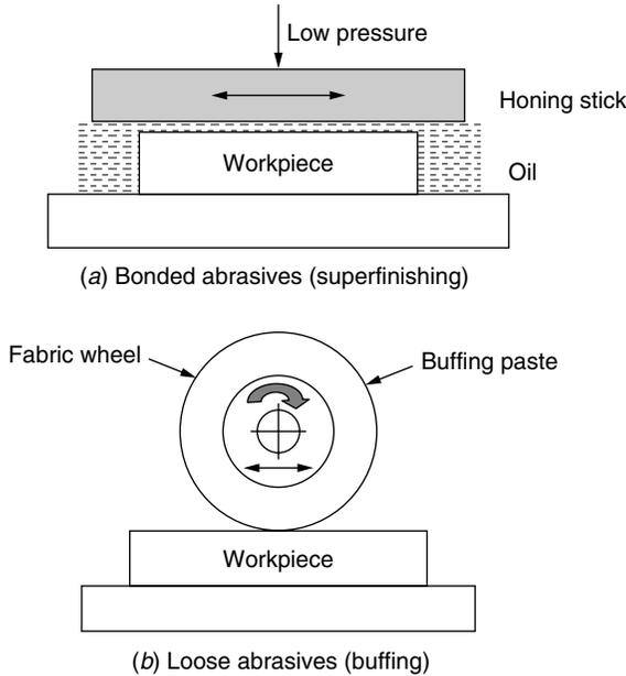
Figure 1.4 Abrasive machining.
