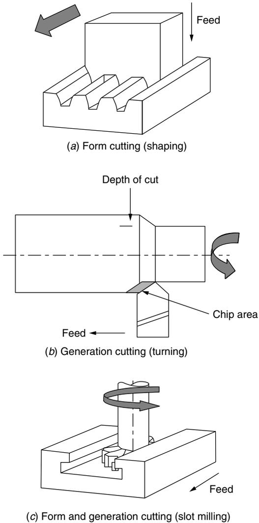
**Figure 1.3** Metal cutting processes.
