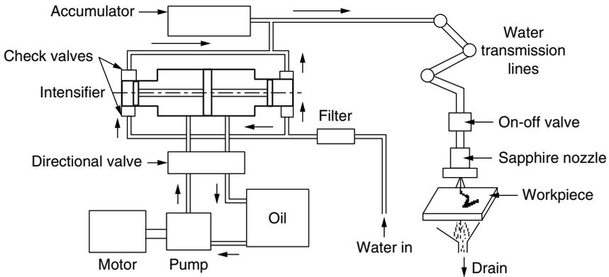
**Figure 2.19** Schematic illustration of WJM system.
