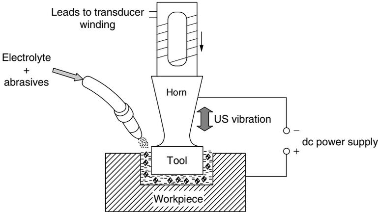
**Figure 6.18** USMEC schematic.
