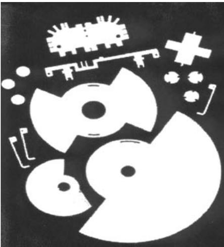
**Figure 3.12** Typical PCM blanks ([www.chemart.com/](http://www.chemart.com/)).
