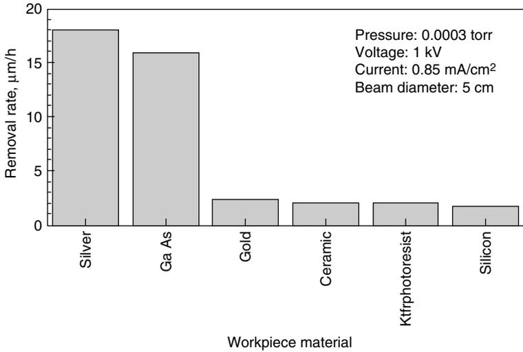
Figure 5.58 Removal rates for different materials (El-Hofy, 1995).
