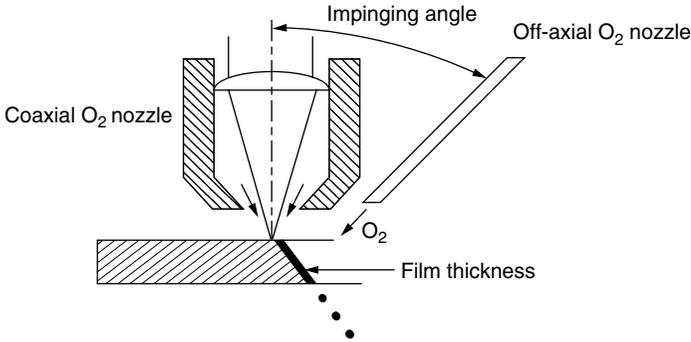
**Figure 5.39** Off-axial gas-assisted laser cutting (Hsu and Molian, 1995).
