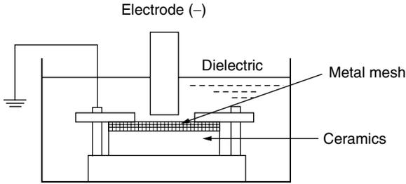
**Figure 5.24** EDM of insulating ceramics (Fukuzawa et al., 1995).
