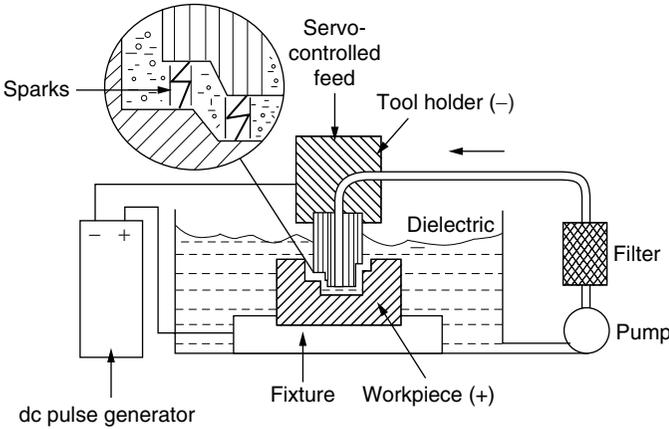
Figure 5.7 EDM schematic.
