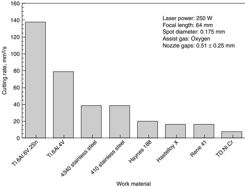
**Figure 5.36** Machining speeds of aerospace alloys in gas-assisted LBM (El-Hofy, 1995).
