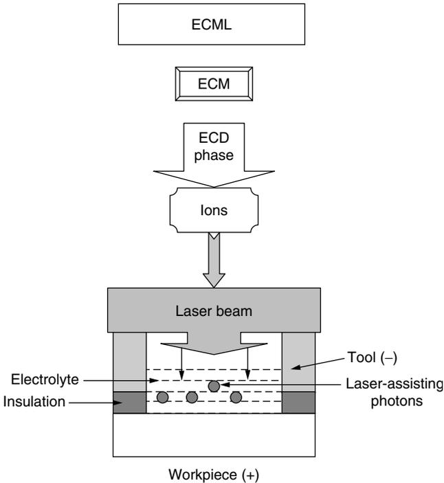
**Figure 6.20** ECML schematic.
