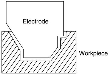
Figure 5.20 EDM die sinking.
