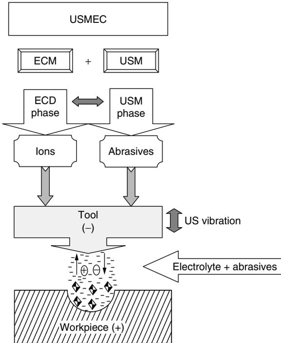
Figure 6.19 USMEC components.
