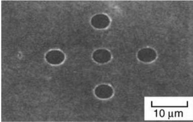
**Figure 5.29** Microholes produced by EDM (Masuzawa and Tonshof, 1997).
