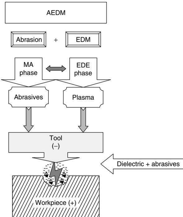
Figure 7.19 AEDM components.
