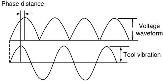
**Figure 7.4** Voltage and tool-oscillation waveform (El-Hofy and McGeough, 1988).
