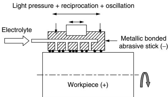
**Figure 6.12** ECS using metallic bond diamond stick (Youssef, 1971).
