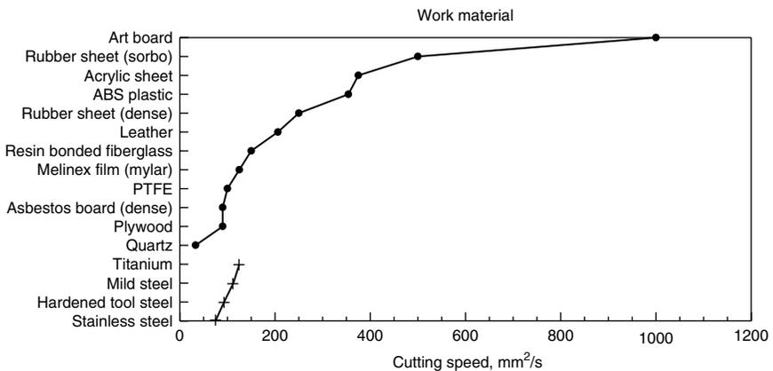
Figure 5.34 Cutting speeds in  $\text{CO}_2$  LBM (El-Hofy, 1995).
