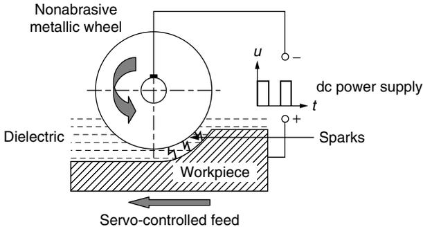
Figure 7.12 EDG schematic.
