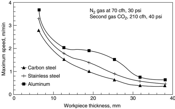
Figure 5.53 Machinability of different material in gas-shielded plasma (El-Hofy, 1995).
