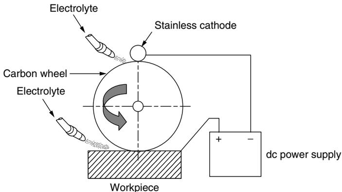
Figure 6.16 ECB schematic.
