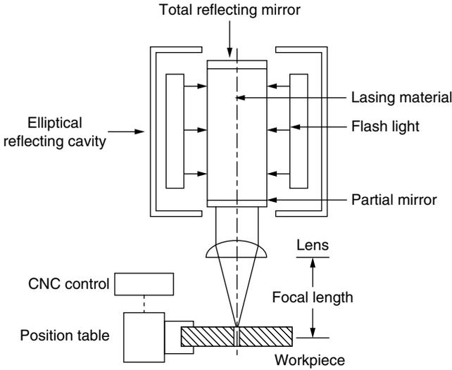
Figure 5.32 LBM schematic.
