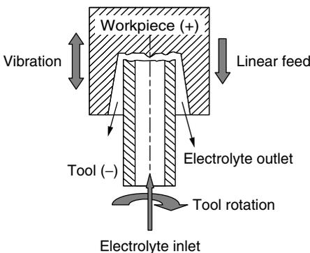
**Figure 7.3** EEDM drilling.
