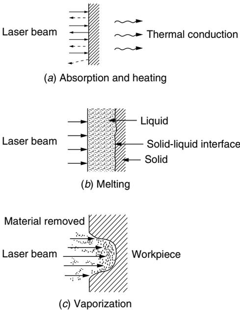
Figure 5.33 Physical processes occurring during LBM.
