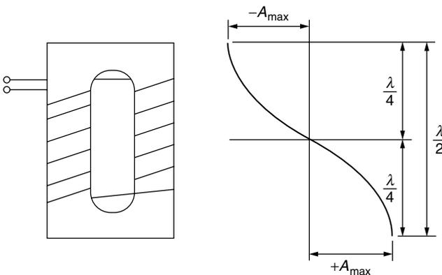
**Figure 2.7** Variation in a wave of elongation along the length of the magnetostrictor (Kaczmarek, 1976).
