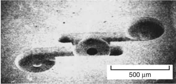
**Figure 2.18** Micro-ultrasonic machined cavity (Masuzawa and Tonshof, 1997).
