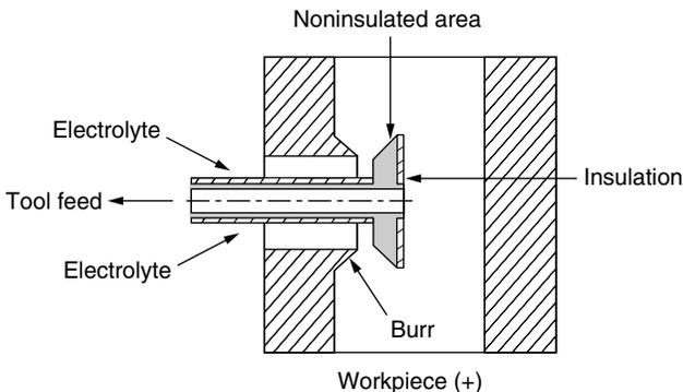
**Figure 4.31** Hole deburring.
