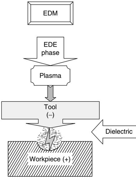
Figure 5.1 EDM components.
