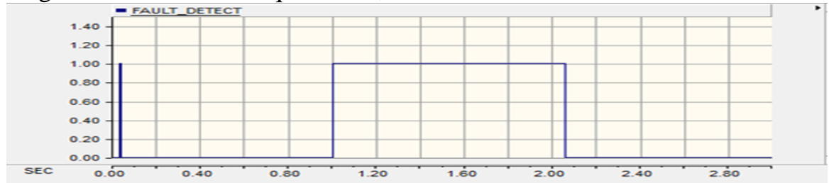
Fig 4-8 internal SCSFCL model component performance (FAULT_DETECT)
