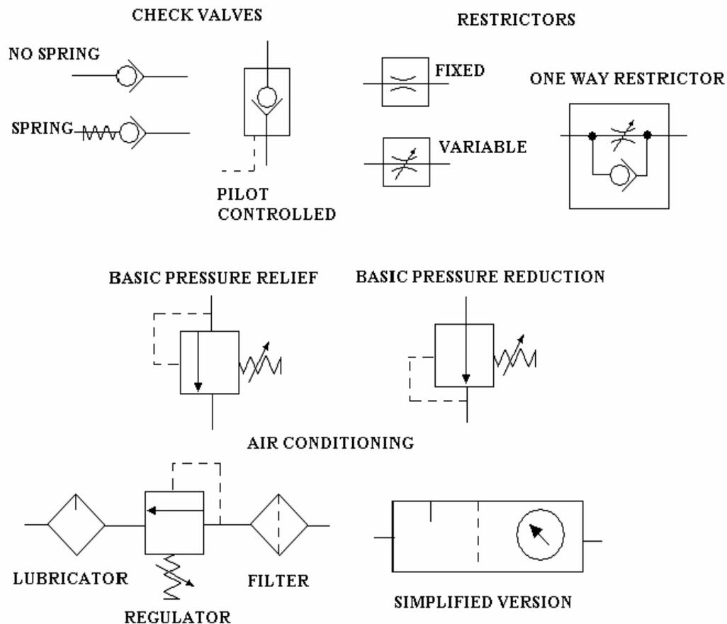
**Figure 2-28 Types of symbols used in hydraulic circuits.**
