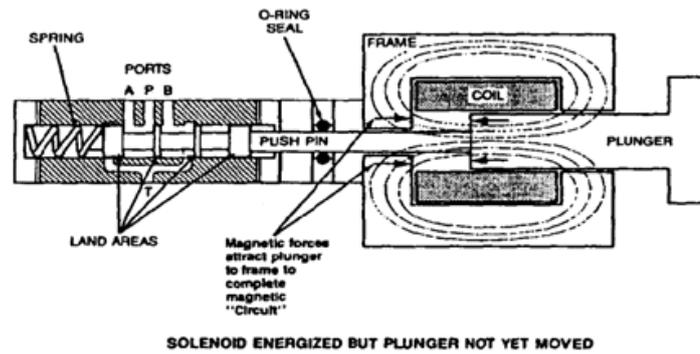
**Figure 2-9 Solenoid operated control valve**
