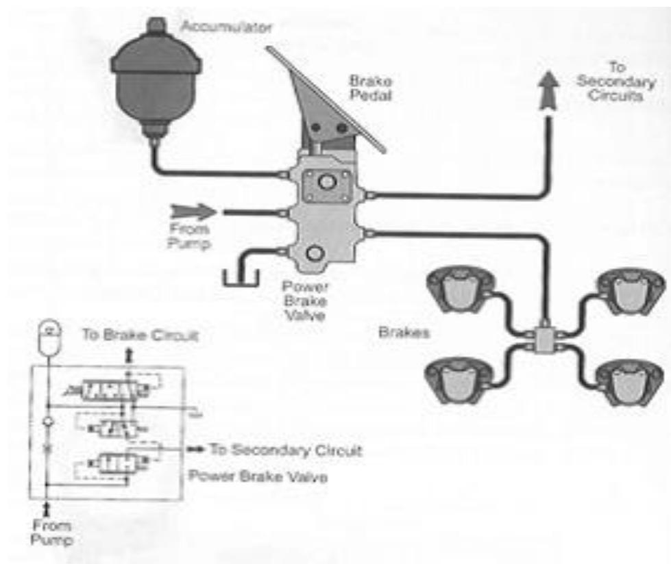
**Figure 2-21 Hydraulic accumulators in brake system.**
