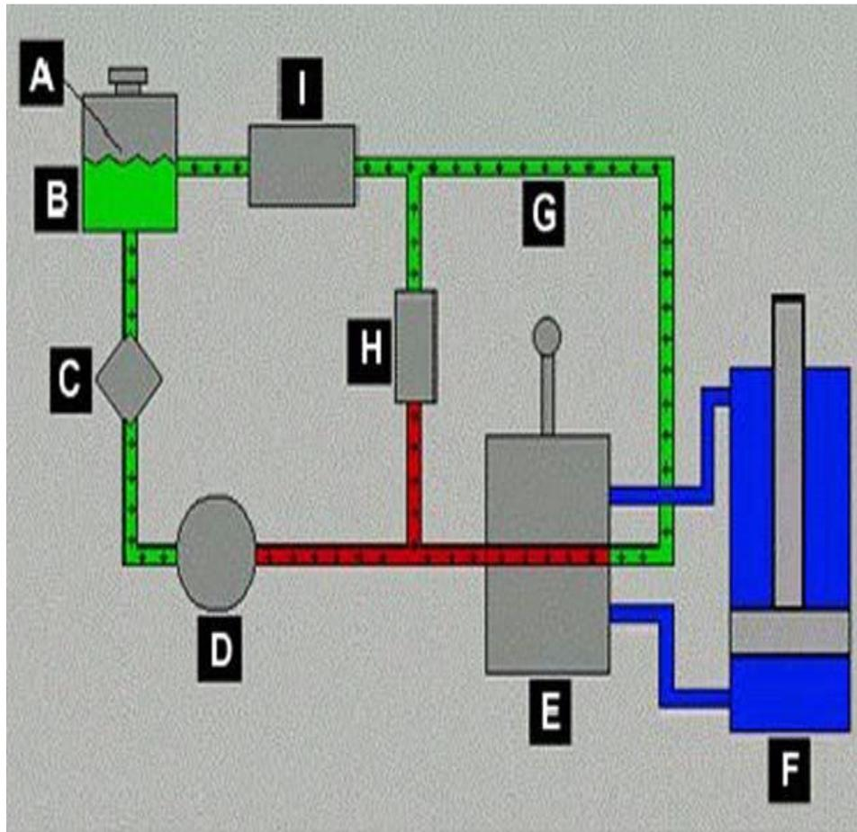
**Figure 2-25 basic hydraulic system components**
