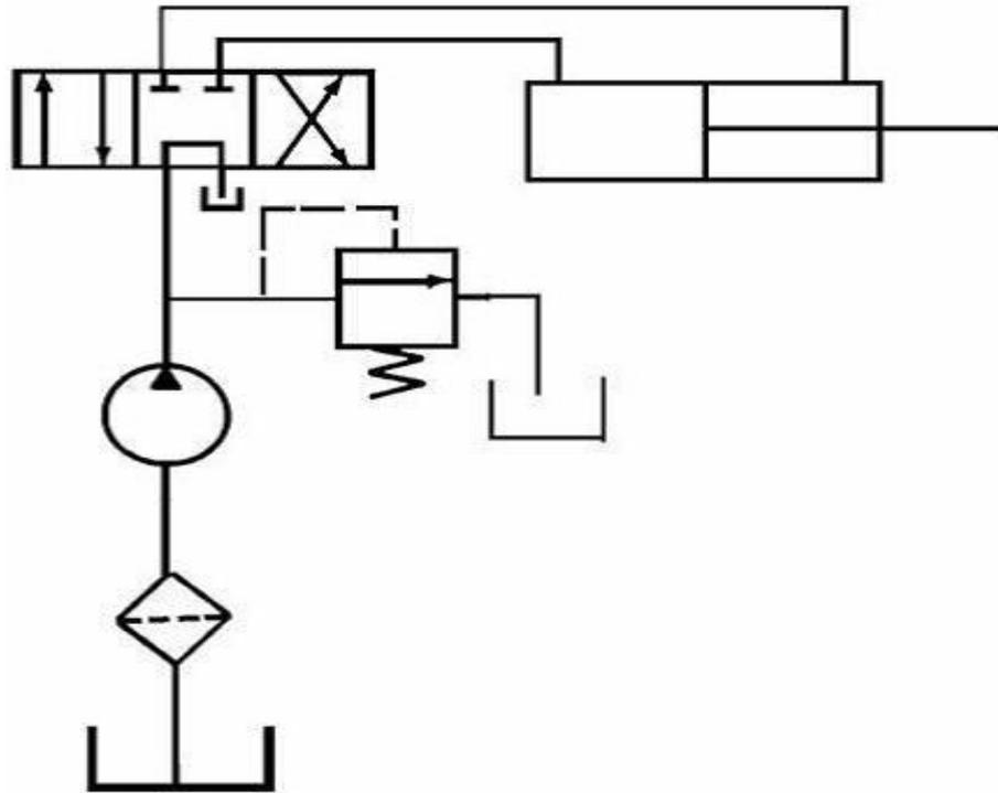
Figure 2-26 simple hydraulic circuit
