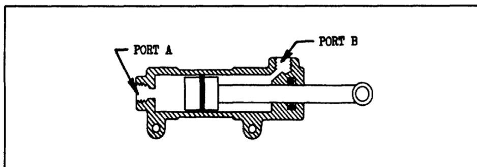
**Figure 2-16** double acting cylinders
