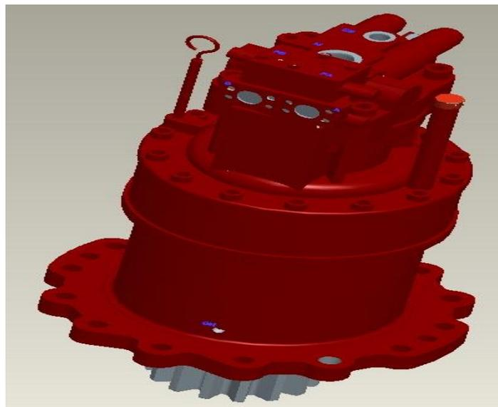
**Figure 2-14 Hydraulic swing Motor**
