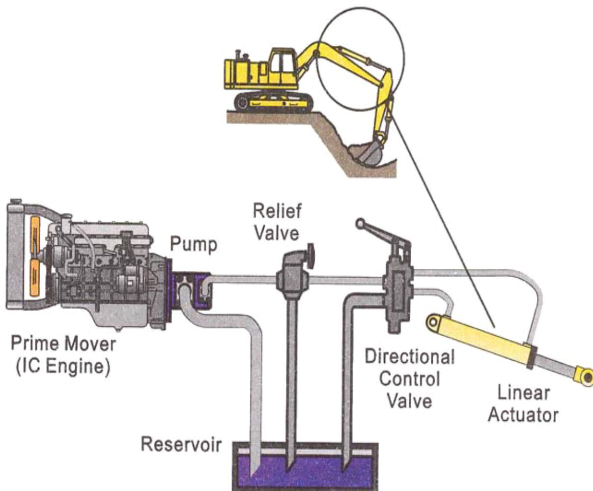
**Figure 2- 2 Excavator hydraulic components**
