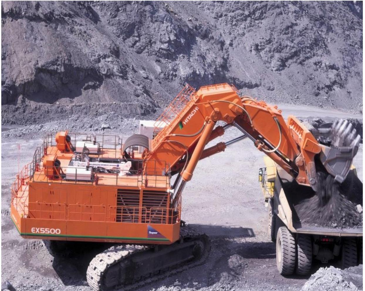
**Photograph 10 Excavator 5500 HITACHI loading Dump truck**
