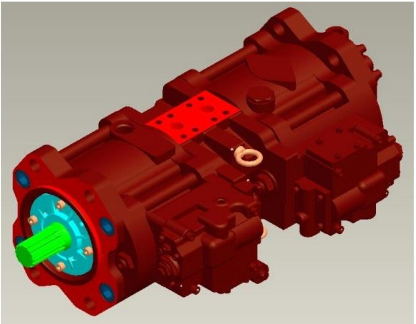
**Figure 2-4 a photograph of the main hydraulic pump and pilot pump**
