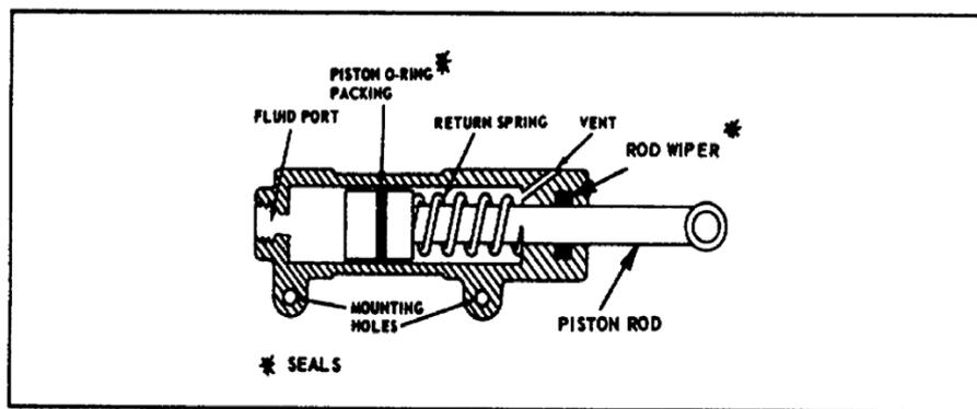
**Figure 2-15** Single acting cylinders
