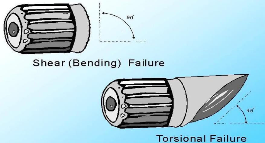
**Figure 3-28 shaft sheared and shaft twisted.**
