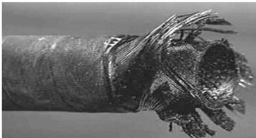
**Figure 3-20 hose Coupling Blow- Off**
