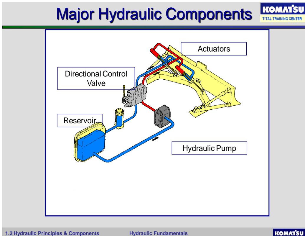
**Photograph 15 - Basic hydraulic components of bulldozer**
