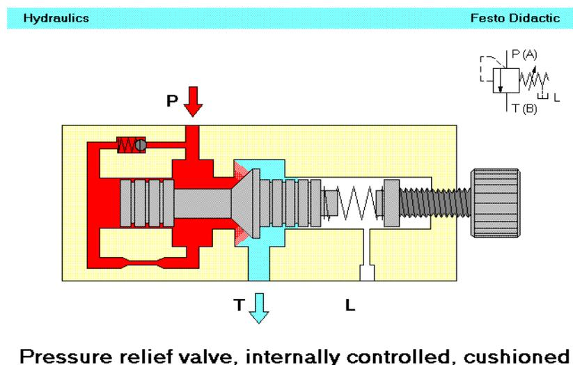
**Figure 2-6 a longitudinal section of a pressure relief valve**
