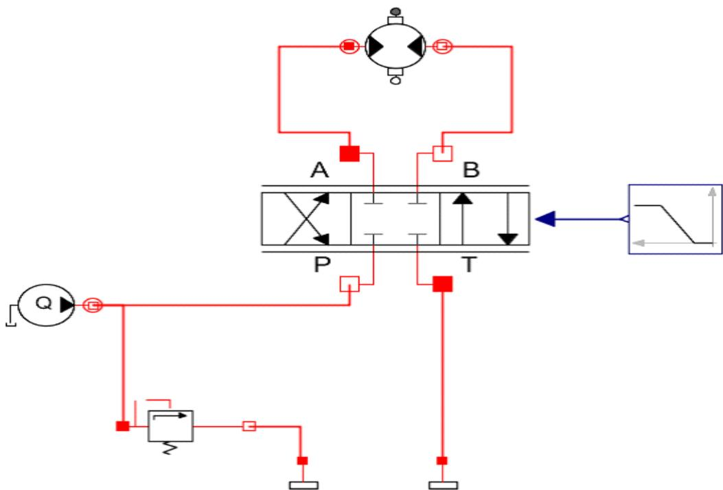
Figure 2-27 Complex hydraulic circuit
