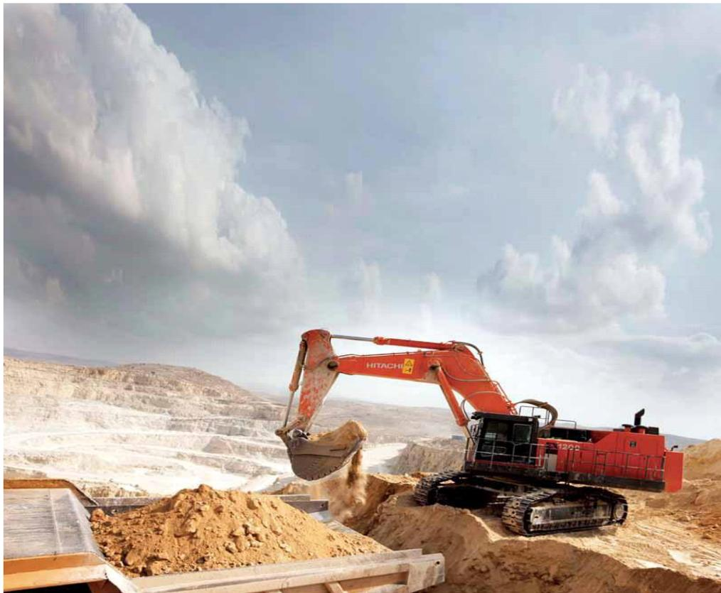
**Figure 1- 2 Surface mining using Hitachi excavators and dump truck**
