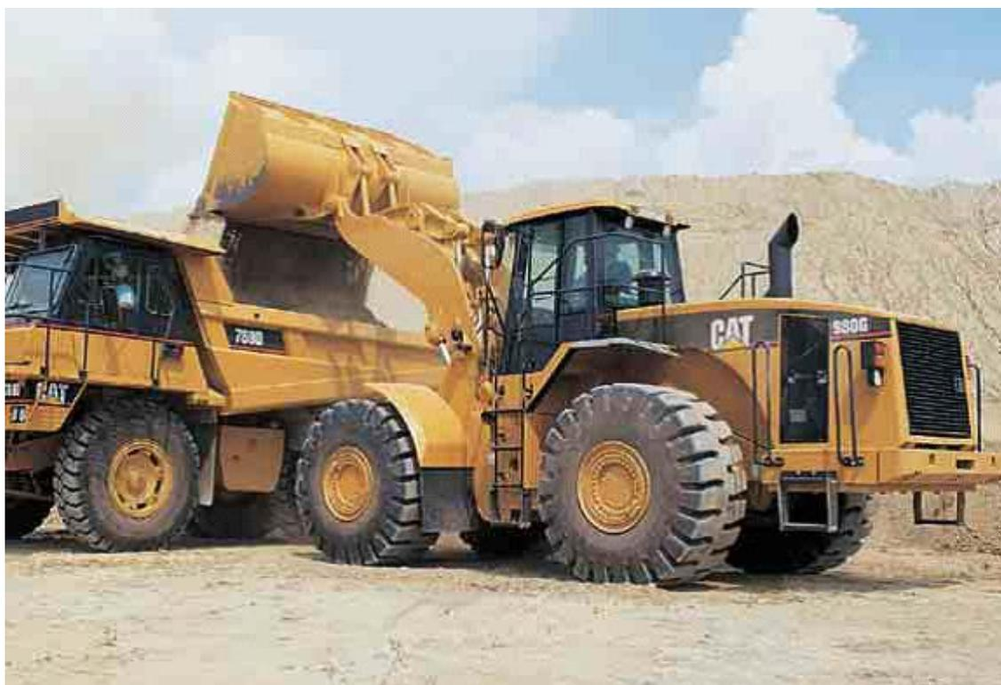
**Figure 1-1 Surface mining using CAT loader and CAT dump truck**
