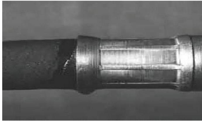
**Figure 3-19 hose leak at thread end**
