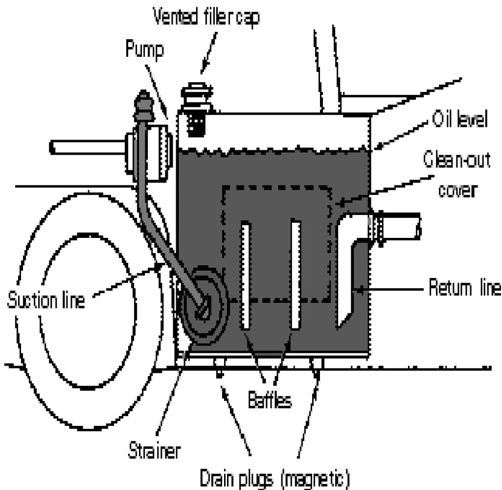
**Figure 2-3 the main components of a reservoir**
