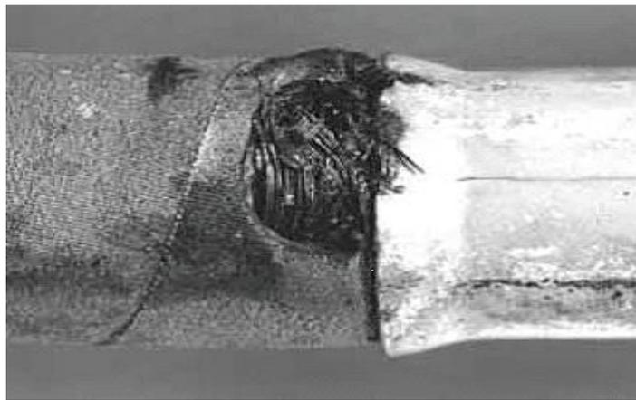
**Figure 3-17 hose burst coupling**
