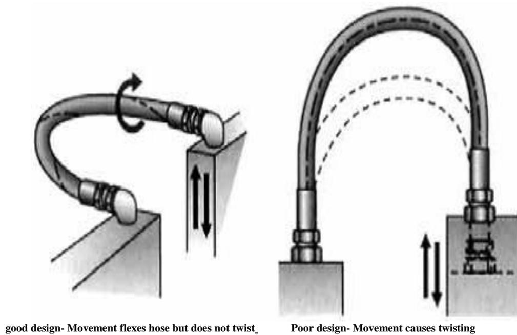
**Figure 2-11 hose poor design twisting and good design not twist**
