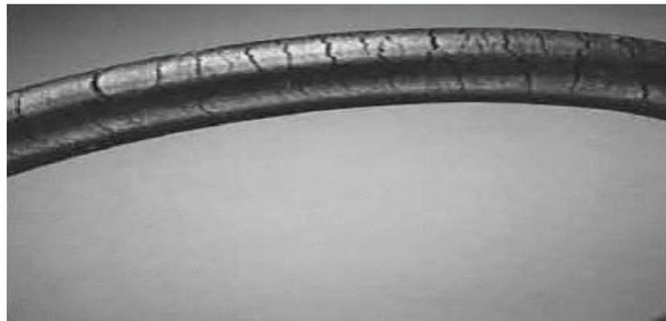
**Figure 3-21 Hose Cracks**
