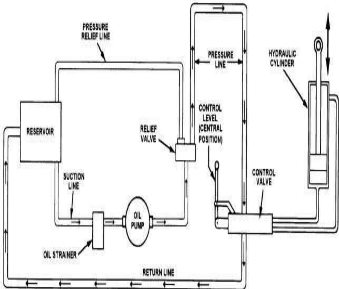
**Figure: 2-1 Basic components of hydraulic circuits**
