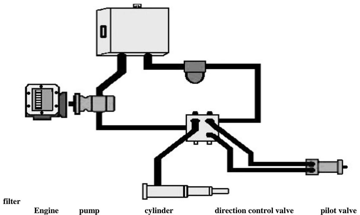
**Figure 3-32 Dump truck hydraulic components.**
