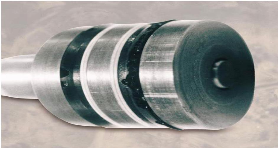
**Figures 3-1 piston rod of bucket cylinder**
