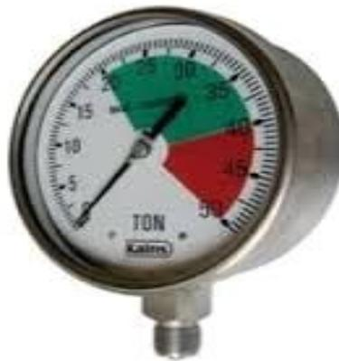
**Figure 3- 8 Hydraulic oil pressure gauge**
