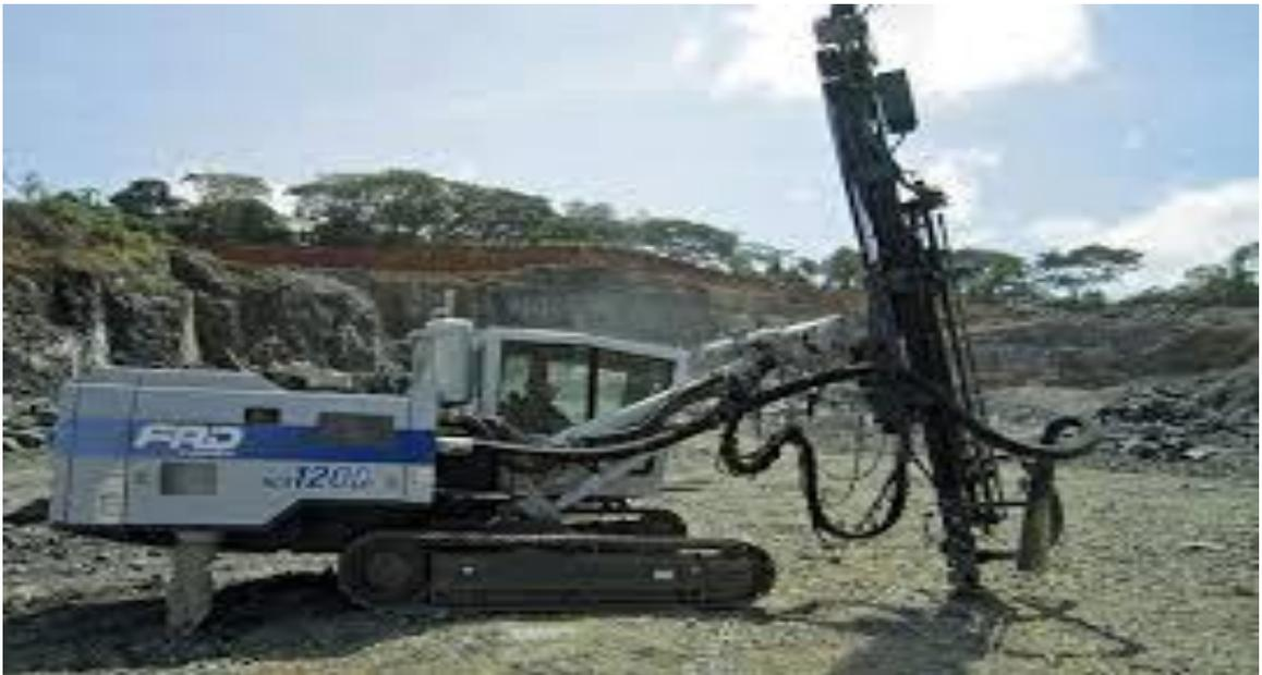
**Figure 3-29 FRD drilling machine which is used in surface mining**
