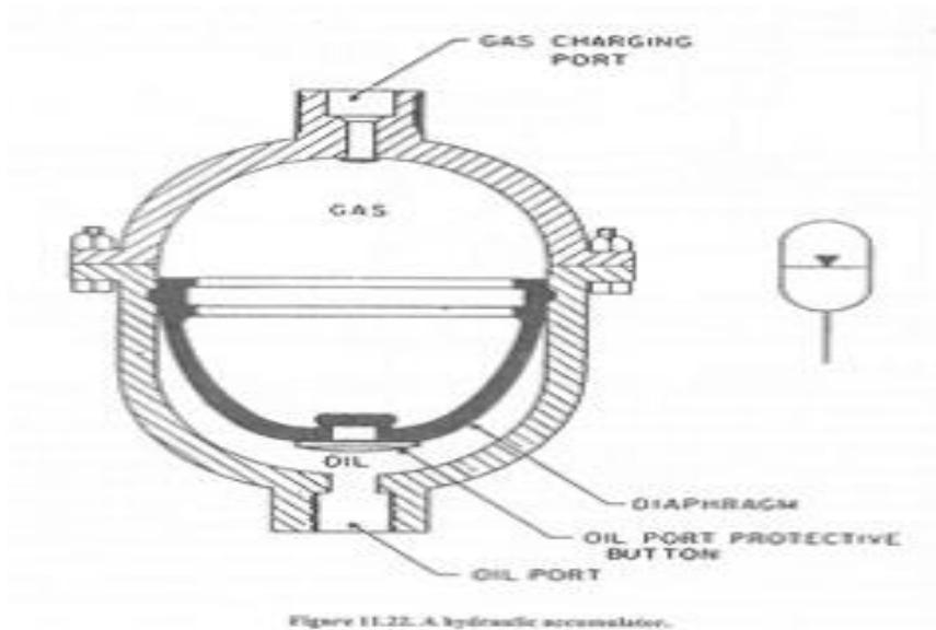
**Figure 2-20 Hydraulic accumulators**
