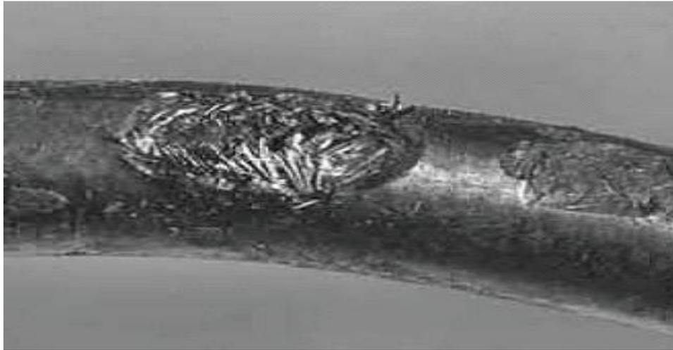
**Figure 3-15 hose damaged by abrasion**
