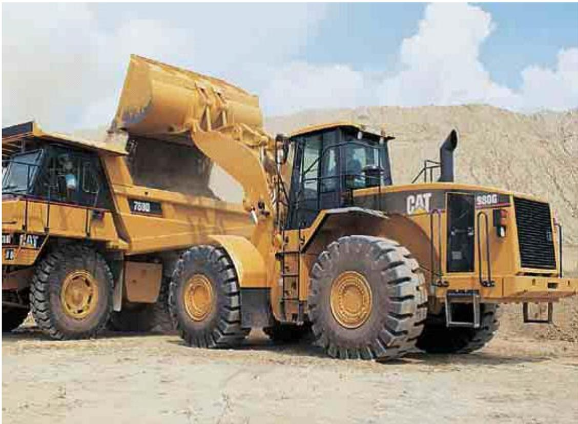
**Figure 3-5 wheel loader 950G- loading dump truck**
