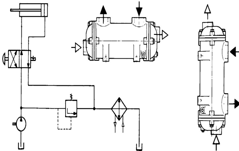
**Figure 2-24 physical representation of hydraulic oil cooler**
