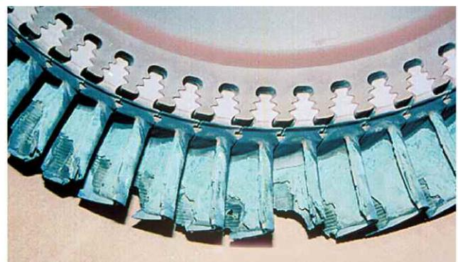
Figure 4. Hot Corrosion on a Turbine Rotor.
