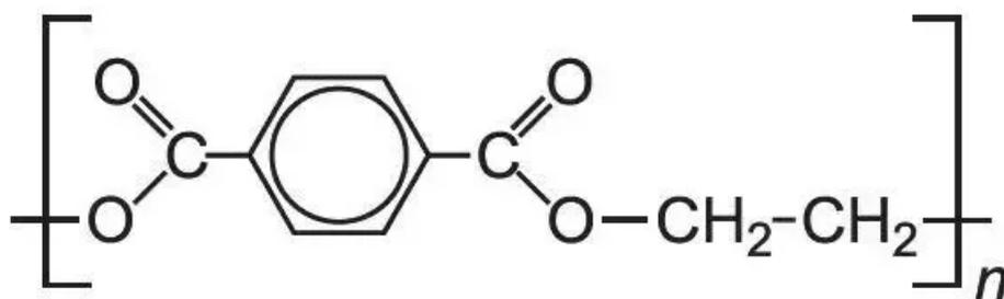
The above substance is polyester. The brackets and subscript 'n' around this diagram representing the fact that this is a single unit of polyester, which is repeated in a chain to create the full fabric. As you can see, there is only carbon, hydrogen and oxygen in polyester (the three elements most common in the human body). The overall structure is reasonably complex, with two standard methyl links, two ester groups, and an aromatic ring (benzene).
