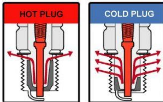
Spark plugs are manufactured with different heat ratings, from very cold to very hot, so a desirable plug can be found for your engine, depending on what you need, based on your riding or driving conditions. Plugs with the same diameter and reach will have different lengths of the insulator nose section and different type numbers to indicate which runs hot and which runs colder.
