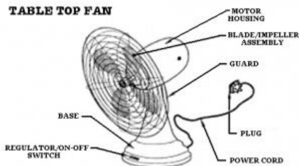
Fans are easy to maintain and repair and can be cleaned easily just because of their simple operational needs whereas a blower might need some serious maintenance efforts as depending upon the application it may or may not be subjected to harsh working conditions and extreme debris and effluents.
