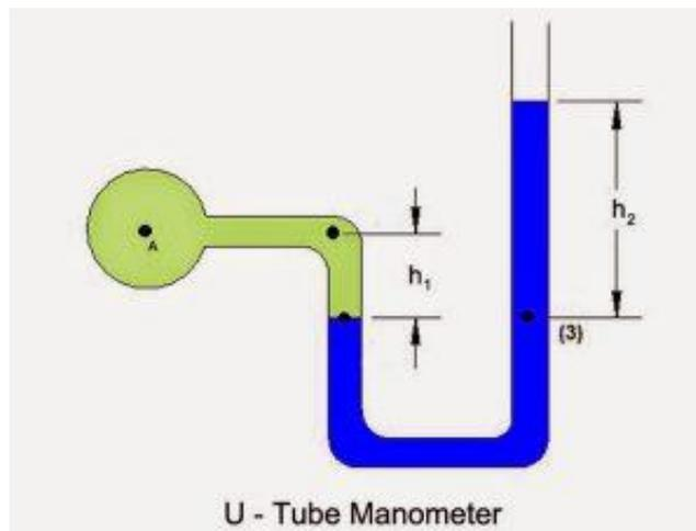
This type of manometer is U shaped, with one end open to atmosphere. It is used for measuring suction. It has the capability of measuring both positive and negative suction pressures. It utilizes the principle of specific gravities for measuring the suction pressure. This type of manometer generally has a liquid whose specific gravity is greater than that of the fluid whose suction pressure is to be measured.
