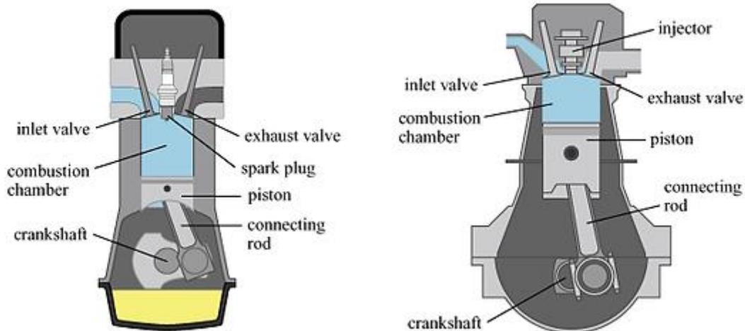
The basic difference between the two is same as that between a petrol engine and a diesel engine. This line is just for you guys to get a small hint of what we are talking about. So here we go.
