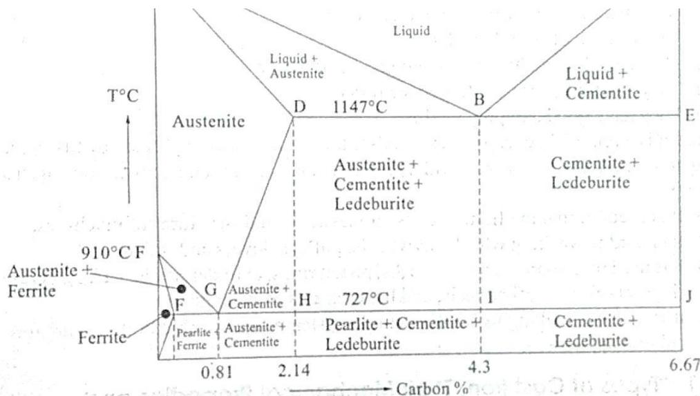
Fig. 1.1 The Iron-carbon Diagram (Simplified)
