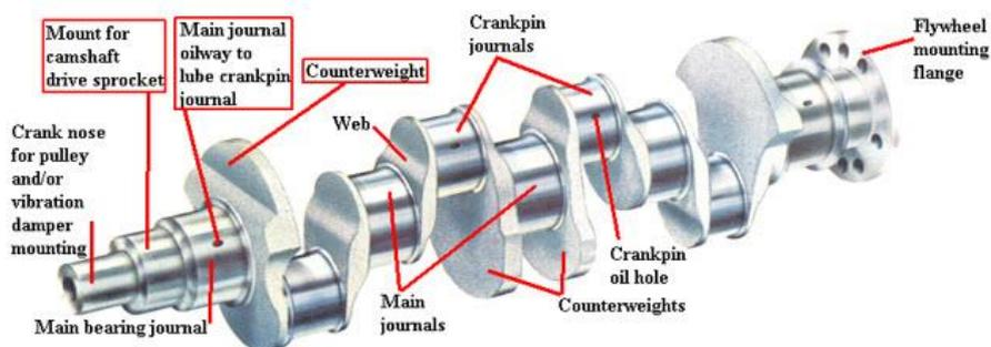
While visually inspecting the crankshaft, you can find the rod bearings are nearly offset or eccentric. Here the offset of the shaft transforms the reciprocating motion (up and down) of the piston in the rotating motion of the crankshaft.
