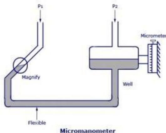
The equation of hydrostatic equilibrium at PQ can be written as
