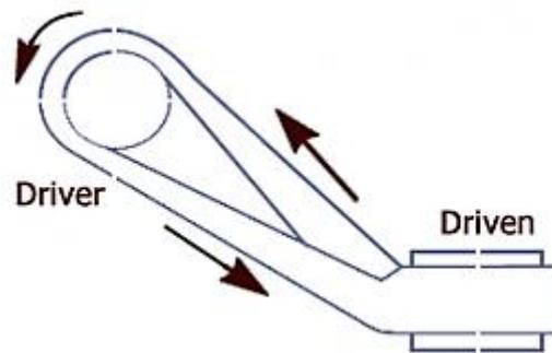
This type of belt drive is also known as right angle belt drive. In these configurations, the shafts are at the right angle and move in one direction. This provides for a unique problem and that is the belt running down the pulley, to overcome this problem the width of the shaft is quarter times more than the width of the belt. Hence the name quarter turns belt drive.
