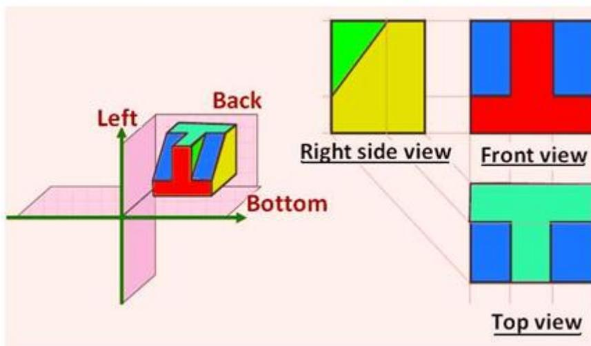
Note that the right-hand side view is projected on the plane placed at the left of the object. After projecting on to the respective planes, the bottom plane and left plane is unfolded on to the front view plane. i.e. the left plane is unfolded towards the left side to obtain the Right-hand side view on the left side of the Front view and aligned with the Front view. The bottom plane is unfolded towards the bottom to obtain the Top view below the Front view and aligned with the Front View.
