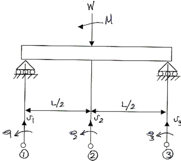
$$\begin{Bmatrix} v_1^1 \\ \theta_1^1 \\ v_2^1 \\ \theta_2^1 \\ v_1^2 \\ \theta_1^2 \\ v_2^2 \\ \theta_2^2 \end{Bmatrix} = \begin{bmatrix} 1 & 0 & 0 & 0 & 0 & 0 \\ 0 & 1 & 0 & 0 & 0 & 0 \\ 0 & 0 & 1 & 0 & 0 & 0 \\ 0 & 0 & 0 & 1 & 0 & 0 \\ 0 & 0 & 1 & 0 & 0 & 0 \\ 0 & 0 & 0 & 1 & 0 & 0 \\ 0 & 0 & 0 & 0 & 1 & 0 \\ 0 & 0 & 0 & 0 & 0 & 1 \end{bmatrix} \begin{Bmatrix} v_1 \\ \theta_1 \\ v_2 \\ \theta_2 \\ v_3 \\ \theta_3 \end{Bmatrix}$$
