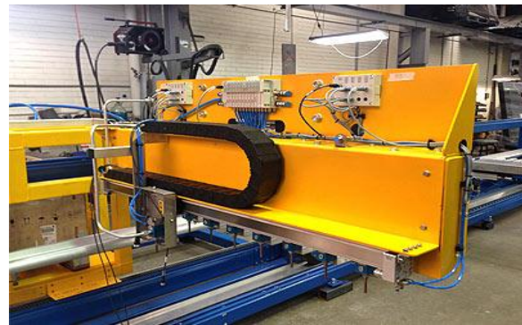
Figure 7. a Special-Purpose Machine used for the Purpose of Material Handling
