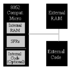
**On-Chip Memory** refers to any memory (Code, RAM, or other) that physically exists on the microcontroller itself. On-chip memory can be of several types, but we'll get into that shortly.
