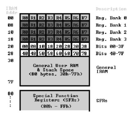
As is illustrated in this map, the 8051 has a bank of 128 bytes of *Internal RAM*. This Internal RAM is found *on-chip* on the 8051 so it is the fastest RAM available, and it is also the most flexible in terms of reading, writing, and modifying it's contents. Internal RAM is volatile, so when the 8051 is reset this memory is cleared.
