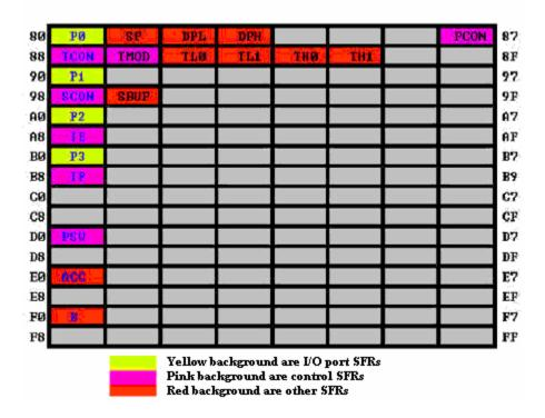
As you can see, although the address range of 80h through FFh offer 128 possible addresses, there are only 21 SFRs in a standard 8051. All other addresses in the SFR range (80h through FFh) are considered invalid. Writing to or reading from these registers may produce undefined values or behavior.
